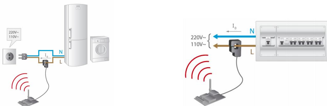
Figures 1 – 2: Smart Metering Wasp mote Plug & Sense! model. Examples of application with the current clamp sensor [12].
